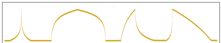
Figure 9: Log and expo shapes generated by patching Env into Time CV and adjusting Rise/Fall CV knobs
